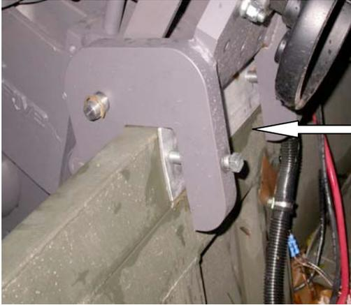
After installing your motor on the boat transom use the aluminum transom saver plate supplied with the unit, torque the bolts to 25 ft. Lbs. Of torque.
