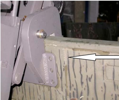
Located on the back of the transom bracket there are three sets of holes on each side. Drill a 7/16" hole through the transom. One on each side in the hole most suited for your boat. Use the 3/8" bolts and nuts supplied with your unit to secure the bracket in the holes drilled.
