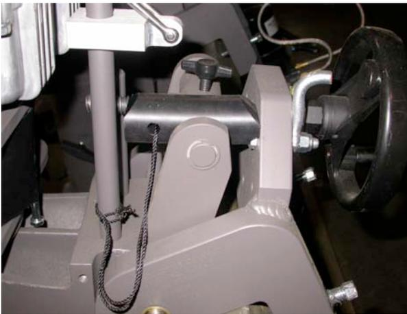
This picture shows the reverse locking block in the lock position.
