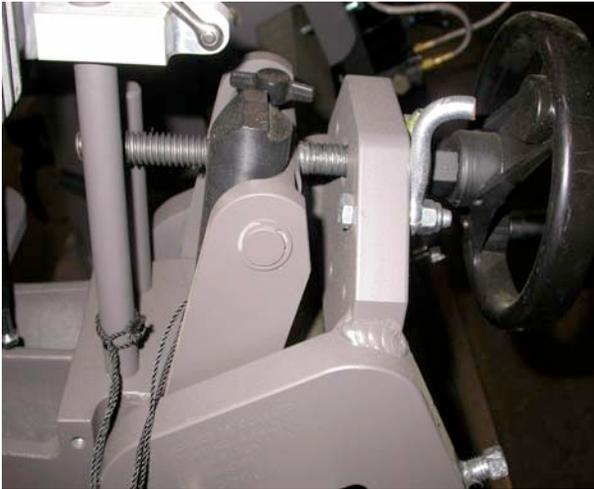
This picture shows the reverse locking block for a manual trim unit, in the unlock position.
