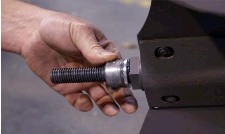
**Install the prop by hand using gloves and tighten thoroughly. It is not necessary to use the wrench for this step. Once the prop is on the shaft, replace the prop nut and tighten by using 1-1/16" wrench.**
