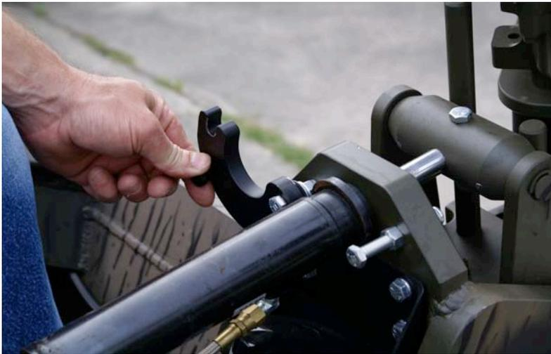
**Step 3. Once the unit is in reverse, lock the trim down with the lever loc.**
