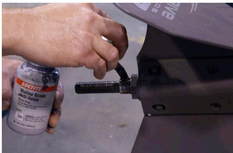
**Install the tapered bushing as shown, making sure that it is fully forward and bottoming out at the threads end. Coat the outside diameter of the bushing as in the above step.**
