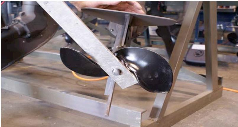
**Remove prop nut using a 1-1/16” wrench or deep wall socket. Next, install the prop wrench as shown . Replace nut to ensure that the prop wrench will not slip off when removing prop. Turn the wrench counter clockwise until the prop is removed.**
