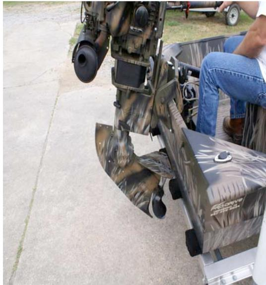
**This picture shows the release lever lock for units with hydraulic power trim in the unlock position.**
